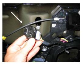
Remove window switch and reconnect. Wire tie switch in safe location.
